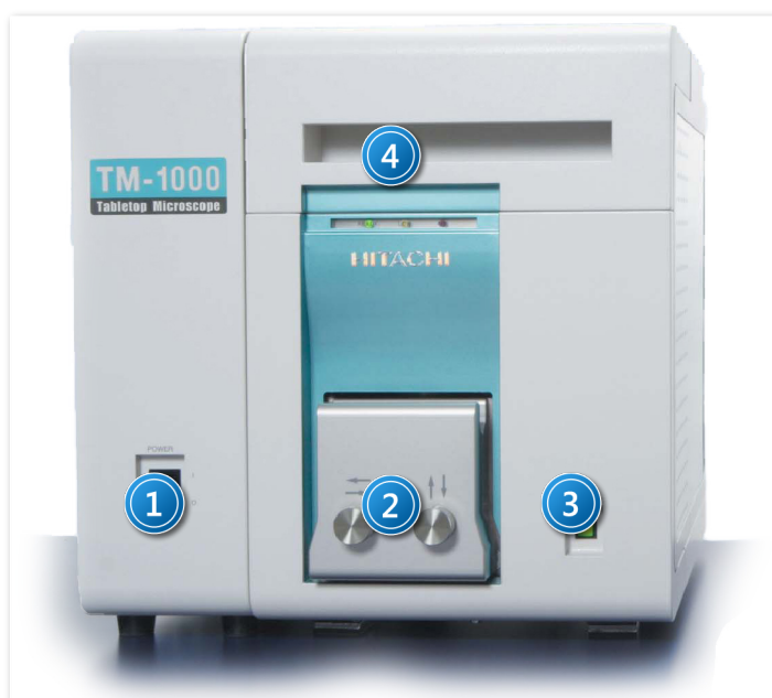
Picture 2. Front view of the TM-1000 microscope: 1 – main switch; 2 –specimen stage; 3 – vacuum mode button; 4 – vacuum state indicator LEDs.
