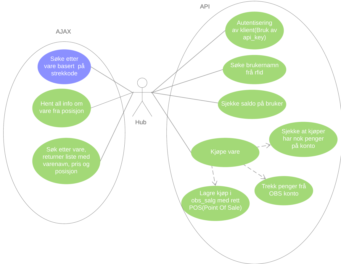
Figure 8: Use case for function the API should have. The blue one is a optional function, and will be implemented if there is time.
