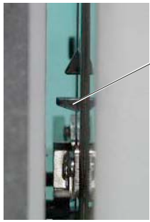
Needle bar height gauge
