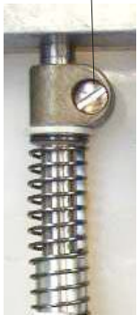
Needle bar holder screw
