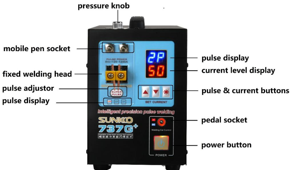
(**Attention:** When the foot pedal is plugged in, it's in MT mode, otherwise, it's in AT mode.)
