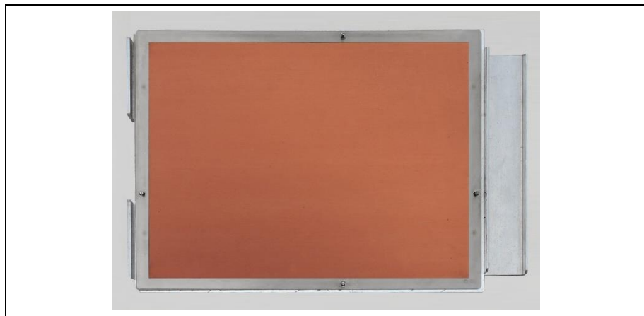
Fig. 318: Copper foil on the lower steel press sheet
