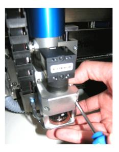
> Connect the camera cable on top of the camera (3) and then connect the cable to the PC. To run the cable, use the free position of cable brackets (4) at the exhaust hose.
