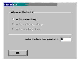
Click on the correct position. If there is not yet any tool within the machine or if the tool magazine is occupied, only click on **OK**.
