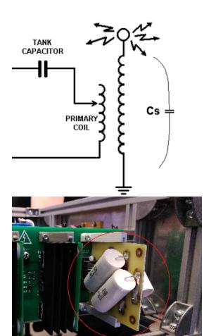
While the inductors can be clearly seen, where are the capacitors in the two LC systems described above? The capacitor in the primary circuit is a "regular" capacitor (serial-parallel bank) located inside the driver chassis ("Tank Capacitor"). For the secondary circuit, the two surfaces of the capacitor are made up of the top load and the surrounding environment ( $C_s$ ).
